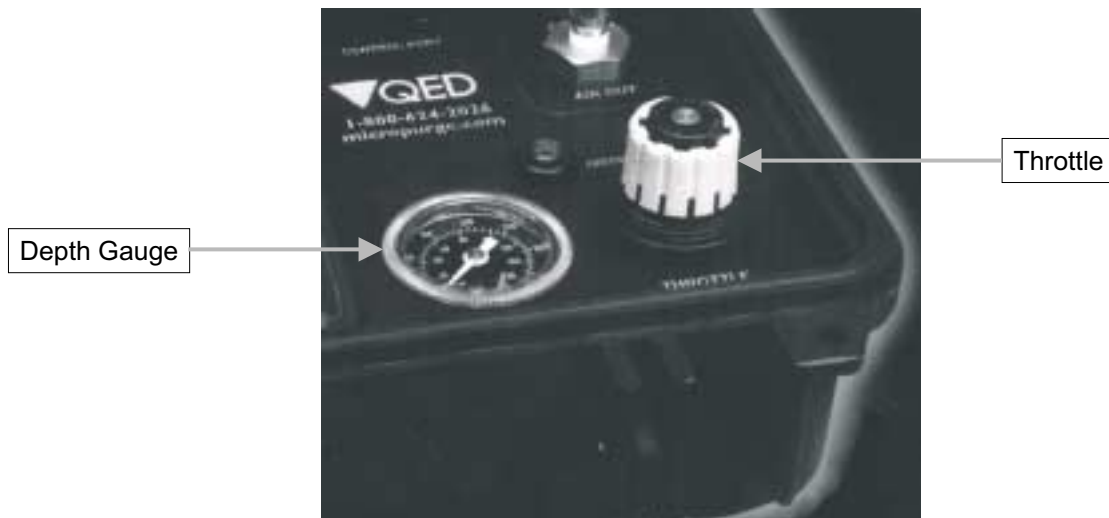
Figure 4 MP10 Throttle and Gauge
